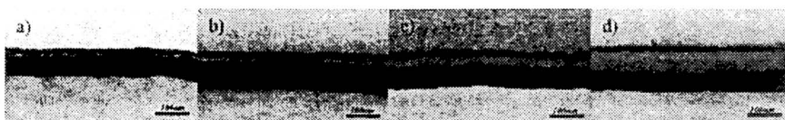
Figure 8. TEM images for (a) 5, (b) 10, (c) 20, (d) 30 bilayer films of PFS-PSS. (Reproduced with permission from reference 33.)
